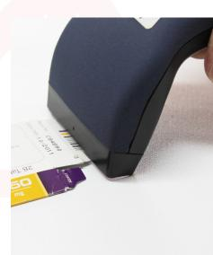
The Axicon 6000W Laetus pharmacode verifier has been specifically designed to meet the requirements for verifying the Laetus pharmacode (commonly called the Laetus or PCE Code) within the pharmaceutical industry. As these codes may be printed in several colours, they cannot be verified by conventional ISO/IEC compliant verifiers, and this special application was created by our engineers. It is a verifier that refers to the Laetus pharmacode specifications for print quality.
